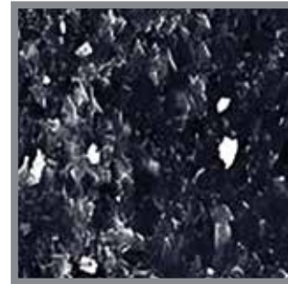
Fractured 321 Grain (Courtesy of 3M™)
